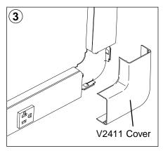
Snap V2411 cover over raceway at corner.
