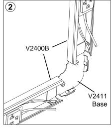
Insert V2400B Base under each tongue of V2411 Base. Mount V2400 Base and Cover per system instruction sheet.
