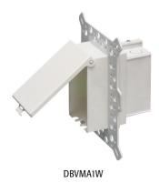
Recessed electrical box with weatherproof-in-use extra-duty cover. Adjustable to fit any foam board thickness. Non-metallic cover and base. Accepts most single gang wiring devices and uses standard indoor wall plates or a GFCI cover plate. Box and white cover are textured/ paintable. UV rated plastic for long outdoor life.
